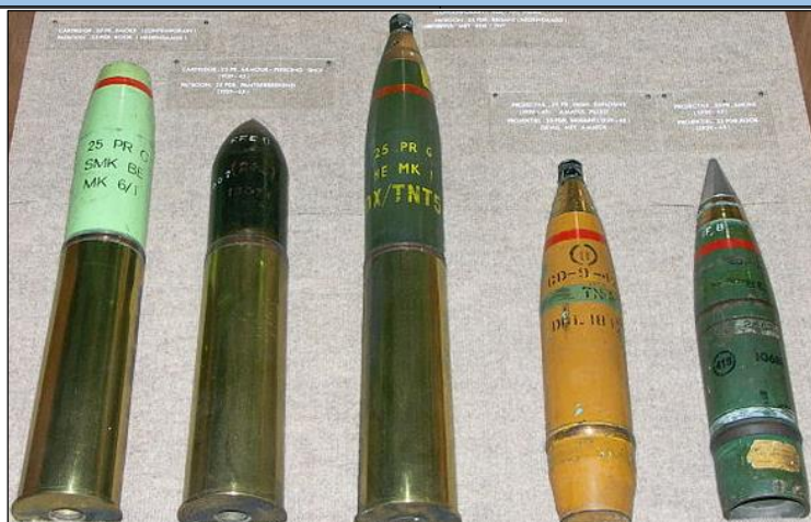
Examples of 25-Pounder shells. From left to right: Smoke, Armour-piercing, HE (RDX/TNT), HE (Amatol), Smoke (WWII)
