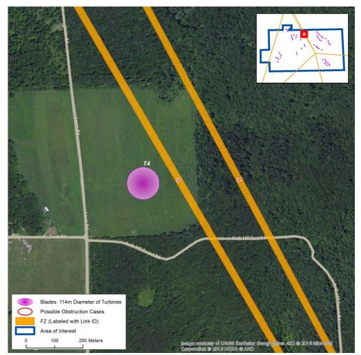
Figure 4: Microwave Paths with Fresnel Zones (turbine T4)
