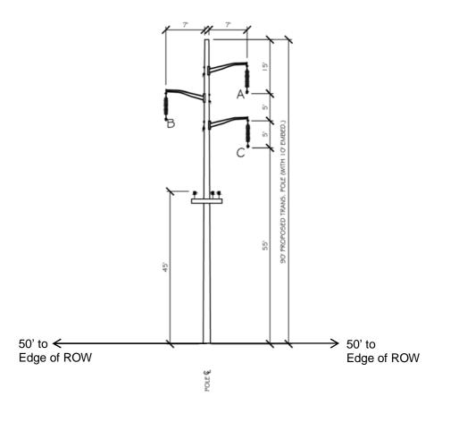
"Typical Proposed 115kV Structure with Underbuilt 34.5kV Collection Line"
