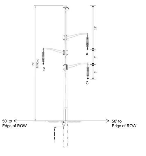
"TYPICAL PROPOSED 115KV STRUCTURES"
