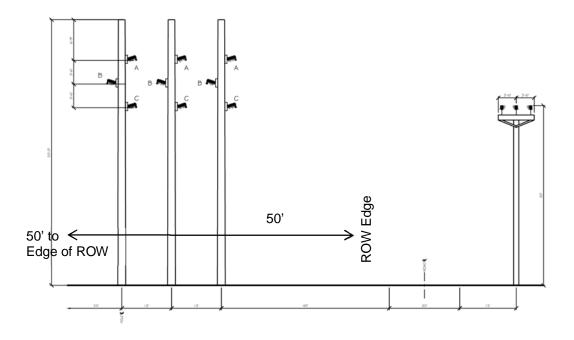
"Typical Proposed (3) 34 kV Collection Structures with parallel Distribution"
