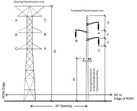
"TYPICAL PROPOSED 115KV STRUCTURE WITH EXISTING 115KV & 34KV"
