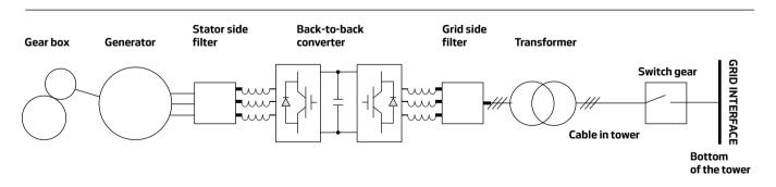
The new power system for the V112-3.0 MW $^{\circ}$  and the V126-3.0 MW $^{\odot}$  enables superior grid support. The permanent magnet generator, coupled with a full-scale converter, meets most challenging grid requirements – in almost any corner of the world.
